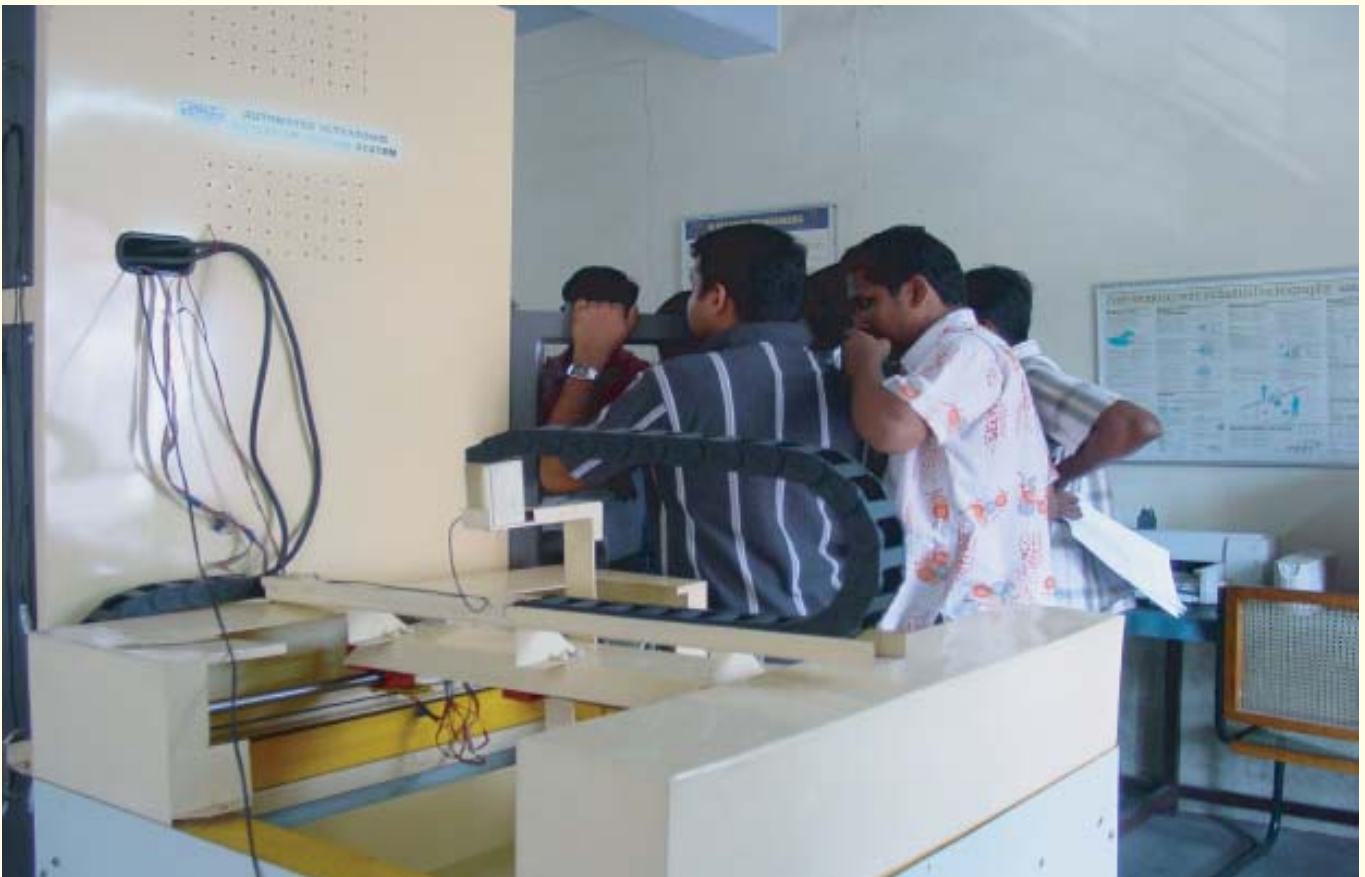
From the Ultrasonic Level I / Level II class. Students are being introduced to the Automated Ultrasonic Immersion Testing equipment.
